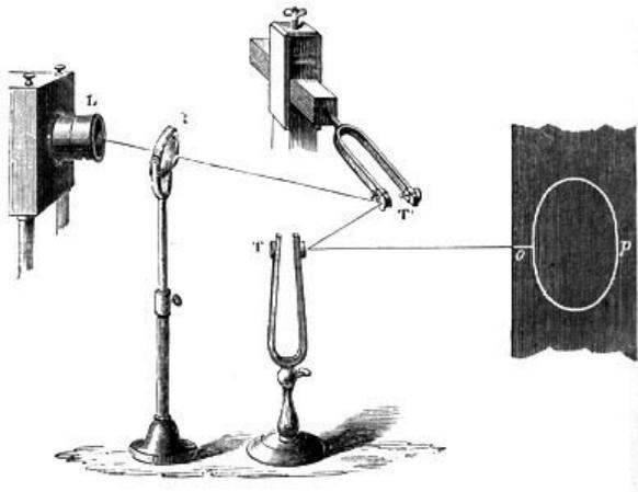
Schematic drawing of Lissajous' machine
